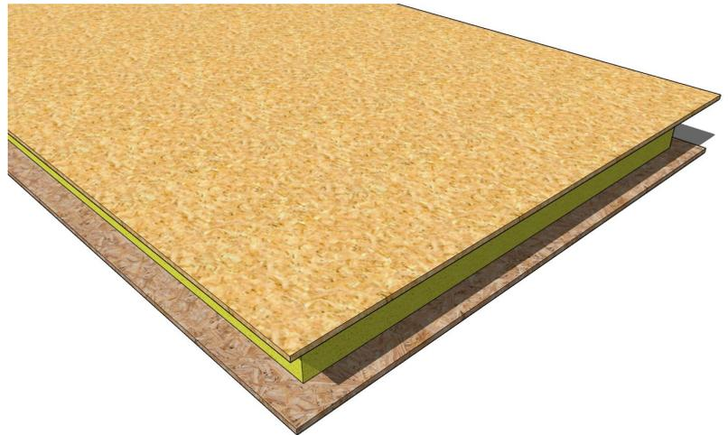
External SURESIP consists of an 11mm OSB-3 internal face and a waterproof 9mm external face with 125 mm rigid polyurethane foam core with a mean density of 40kg/m<sup>3</sup>. At 125mm the U-Value is .17W/m<sup>2</sup>.K compliant part L 2019 building regulation. Use the 152mm External SURESIP when considering floor applications.
